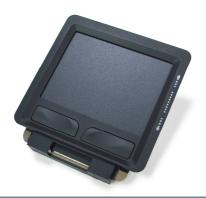
*TPM-3000* TouchPad Module is a pointing device that includes two switches, left button and right button. It also features an emulated scroll wheel of a mouse. To move the cursor, the user can just lightly slide on the device surface by finger. Thanks to modularize mechanical design, it provides flexible product configuration and easy maintenance.
